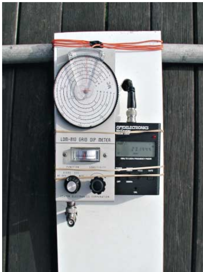
Fig 2. The G3LDO MK4 antenna element resonance measuring kit being used to measure a length of aluminium tube, which gave a half-wavelength of 23.144MHz. The coil is wound directly onto the supporting board above the dial. The G3ZOM circuit has a facility for direct connection to a frequency counter.
